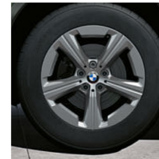
17" light alloy wheels Star-spoke style 832 Light Grey, wheel size 7J x 17 with 205/65 R17 tyres.
